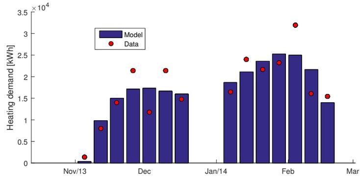
Figure 3: Heating demand (data vs. model).
