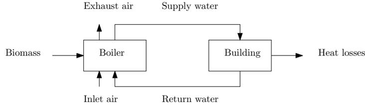
Figure 1: Layout of the physical system.
