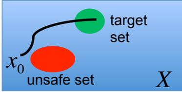
Fig. 1. The probabilistic reach-avoid problem is concerned with finding the probability that the state trajectory, starting from a given initial condition  $x_0 \in X$ , will reach a target set while avoiding an unsafe set.
