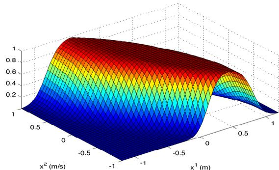
Fig. 2. Probability of reach-avoid for the relative position and velocity of the quadrotor with respect to the ground vehicle.
