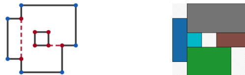
(a) An orthogonal polygon with one hole, 7 convex vertices (blue), 7 non-convex vertices (red), and 2 non-intersecting chords (red). (b) A minimal decomposition of the polygon into five rectangles.
