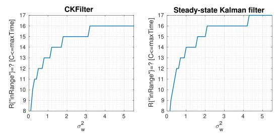
Fig. 7. Expected number of states in which the innovation falls between two standard deviations of the mean.
